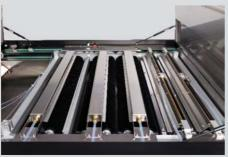
· Constant solvent temperature thanks to water circulation serpentine
