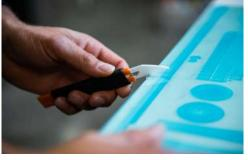
4. Trim all the edges using the Polymount burr trimmer. Do not use any force and hold the trimmer at a 45° degrees angle.
