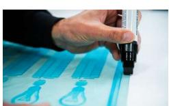
6.1 Apply a thin layer of Polymount Edge Marker along the leading edges. Let it dry for ca. 1 minute.
