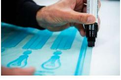
7. Start mounting the Polymount Self-Adhesive sleeve. After mouting please inspect the sleeve and make sure there is no air/ bubbles trapped under the plates.
