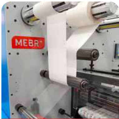
Lamination Station with or without liner
